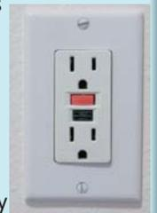
Check for or install ground fault circuit interrupters (GFCIs). A GFCI is an inexpensive electrical device that shuts off power instantly if there is a problem. GFCIs should be installed in all "wet" areas of the home such as bathrooms, kitchens, and basements. GFCIs should be tested monthly to ensure they are working properly. The Consumer Product Safety Commission estimates GFCIs could prevent more than two-thirds of the roughly 300 electrocutions that happen each year in the home.
